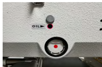
Oiling of the upper shaft is digitally controlled so only a minimal amount of oil is needed.
