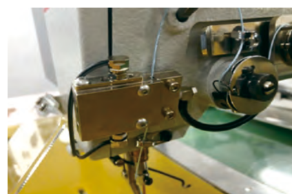
Stitch error detection option (skipped stitches, thread breaks)
